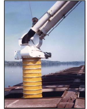
Pivoting gimbal allows different loading angles.
