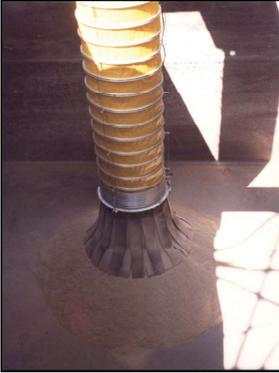
Dust free grain loading into barges.
