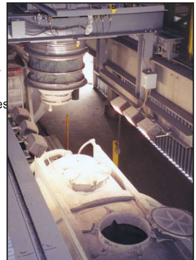
Articulating arm positioning system.
