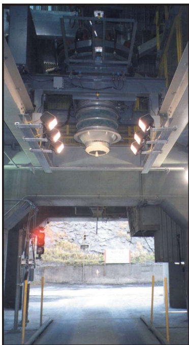
Typical equipment arrangement for fully automatic loading.
