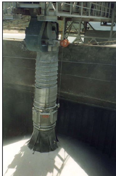
Fig. 4a. Dust free loading is accomplished with a unique design "dead fall" discharge device.
