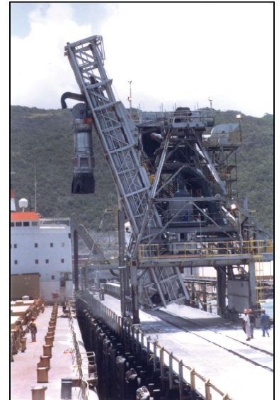
Fig. 2b. Boom and loading spout in stored position.
