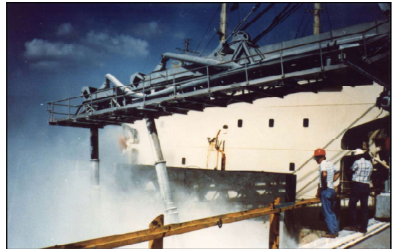
Fig. 2a. Boom in loading position with telescoping conveyor, fully extended.
