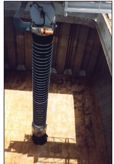
Fig. 3a. Loading spout extends to reach ship hold bottom.
