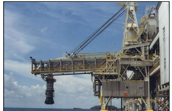
Model OV58 with combination boom and telescopic airslide for alumina loading.
