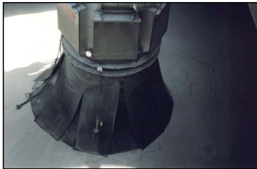
Fig. 3b. Tilt probes automatically raise the spout, with the product pile.
