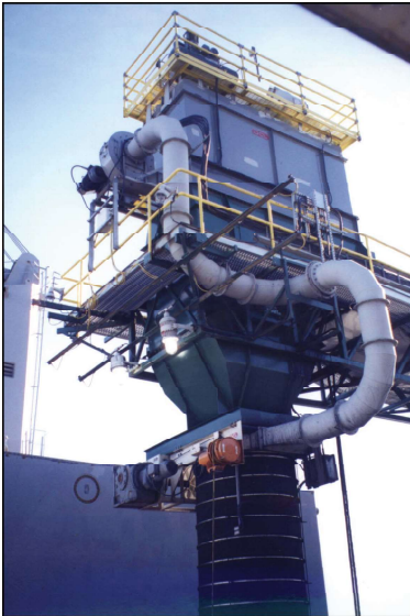
Model OV58 shown w/unique DCL dust collector integral w/ belt conveyor headchute.
