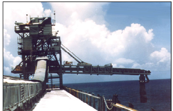
Fig. 2a. Boom in loading position with telescoping conveyor, fully extended.
