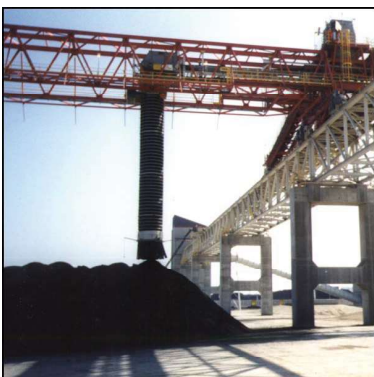
Stockpiling of coal with use of a tripper conveyor.
