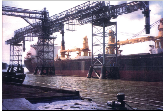
Multiple spout loading system for loadout of calcined coke.
