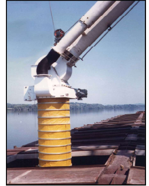
Pivoting gimbal allows different loading angles.
